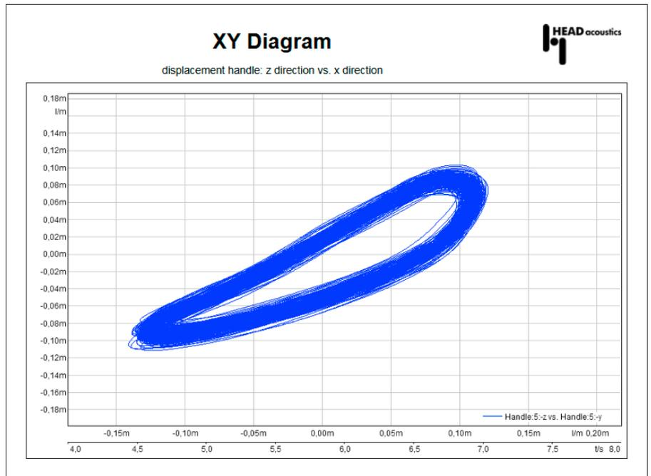
Example of an XY diagram in a report. The XY diagram shows the representation of the deflection during a vibration measurement (z-deflection vs. y-deflection). By zooming, the desired temporal segment can be selected from the relation of the two channels.
