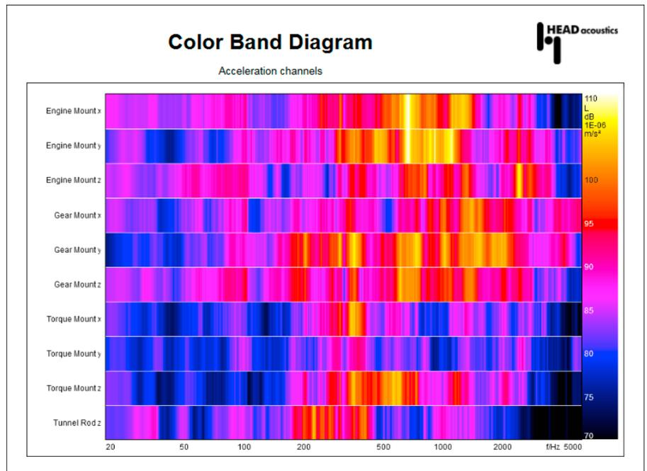
The Color Band Diagram is used for pseudo 3D representation of time signals and 2D analysis results in a report.
