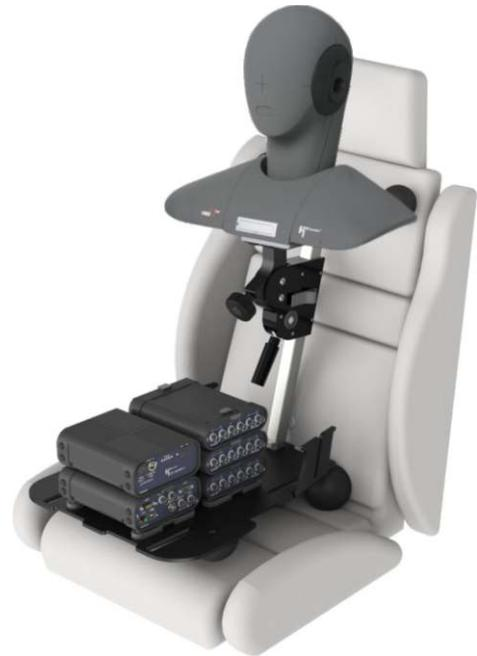
Seat mount adapter HSM V with measurement equipment
