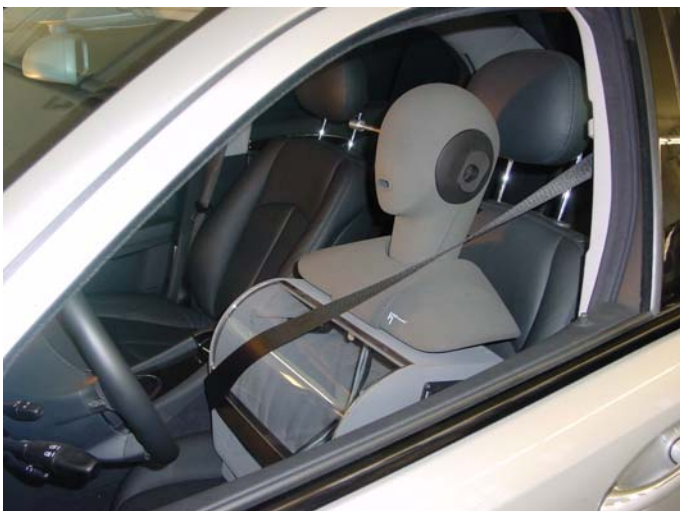
Speech quality tests of car hands-free systems with HMS II.3
